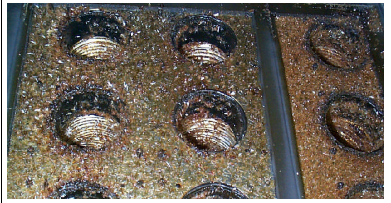
Figure 3: Flux accumulation within the condenser tubes after 30 days and processing of 56.0 kg of solder paste.
